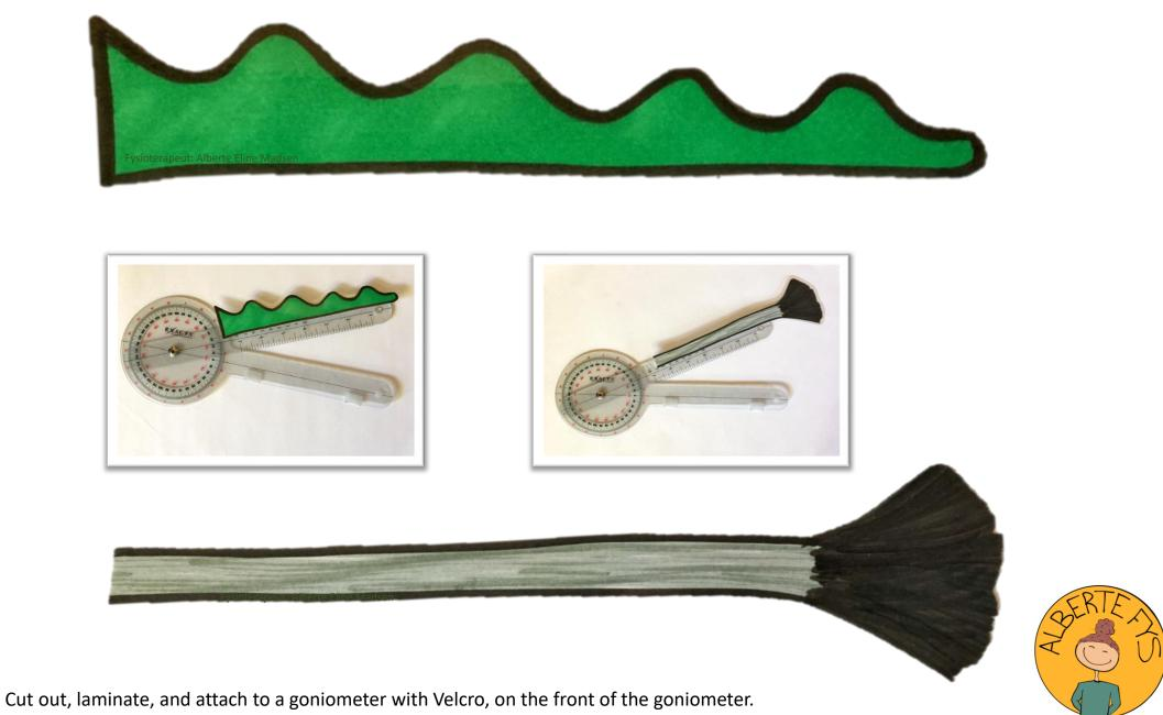
You must be careful not to obscure the two black straight lines on the goniometer, otherwise the measurements will be too imprecise.
