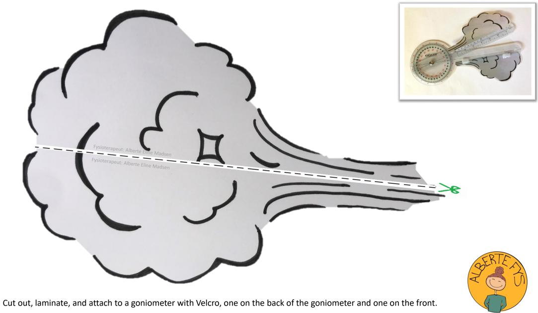
You must be careful not to obscure the two black straight lines on the goniometer, otherwise the measurements will be too imprecise.
